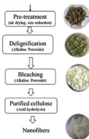
Fig 1. Diagram of the method to get cellulose nanofibers from lignocellulosic filaments [4].
