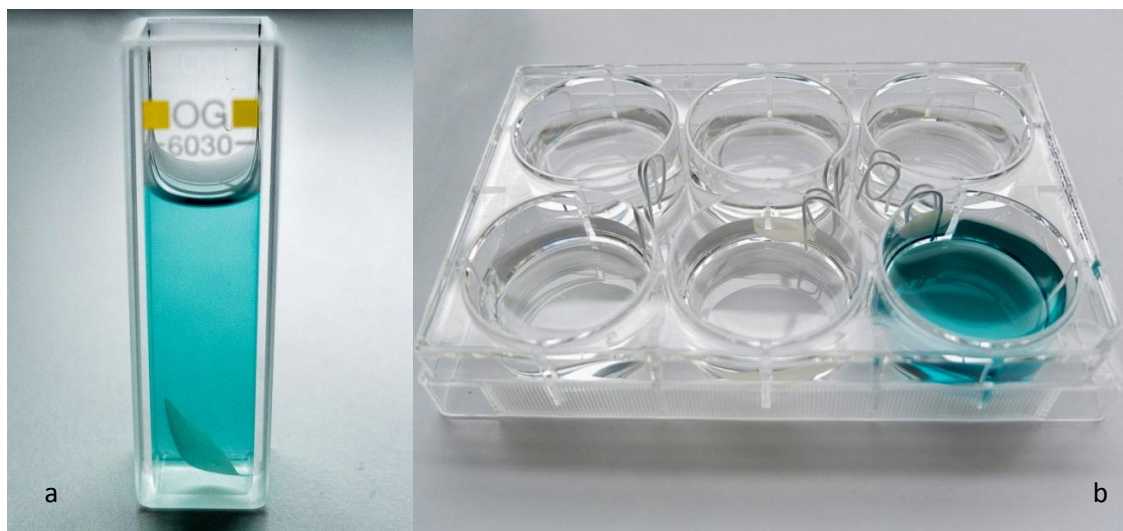
Figure 2 Measurement of the catalytic activity of the immobilized laccase using a cuvette (a) and a 6-well plate (b)
